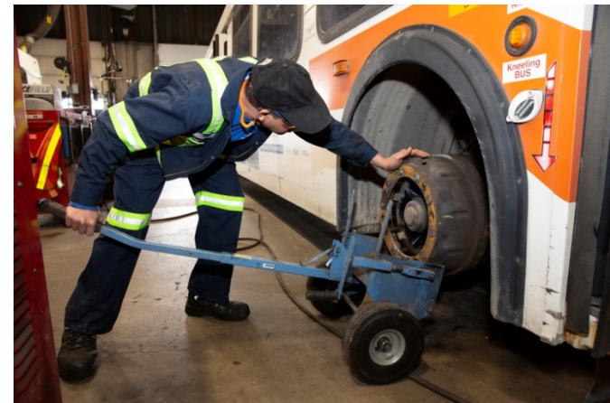
Performing maintenance on a MiWay kneeling bus All MiWay buses are kneeling buses
