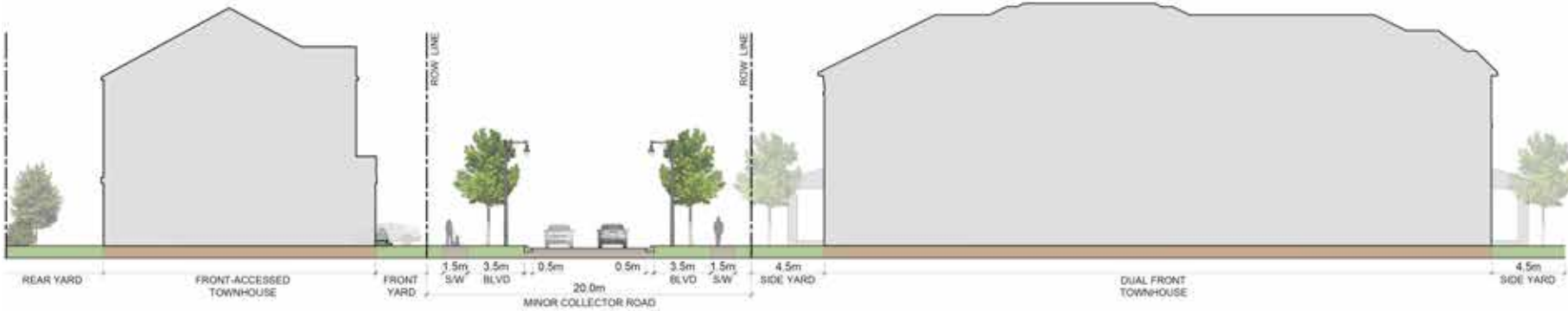
Figure 2.1k - Section B: 20m minor collector entry road interface with front-loaded and dual front towns
