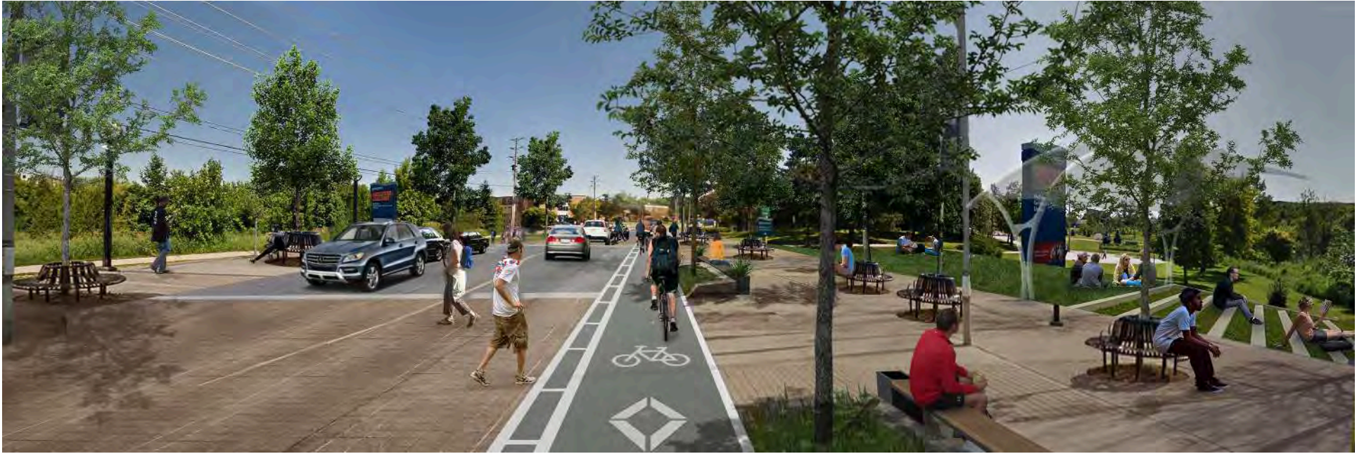
FIGURE 3.9 - Morning Star Drive (after): Pedestrian improvements can be achieved through the use of distinct material treatments that indicate pedestrian crossing areas, as well as the addition of separated bicycle lanes and new street furniture such as public benches.
