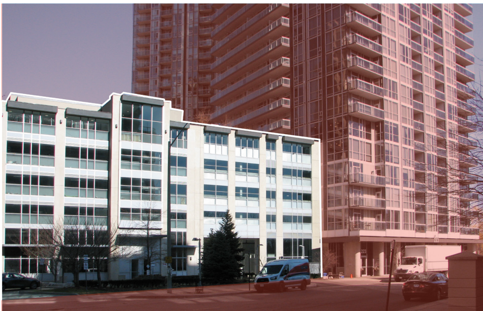
Figure 28: To animate the public realm, a 'vener' (liner buildings) of uses are located between the parking structure and street space to conceal the parking structure (from behind) as part of an integrated development. Downtown Mississauga, Confederation Pkwy & Webb Dr
