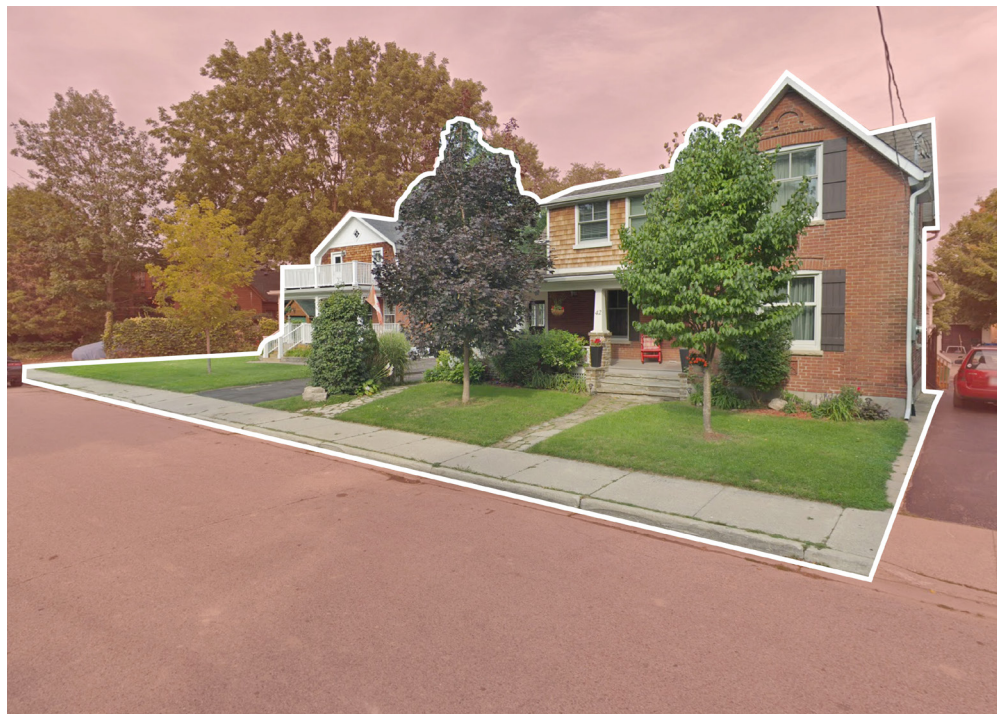
Figure 35: Residential setbacks should be well landscaped. Setbacks should be a minimum of 4.5 m and a maximum of 7.0 m. Mississauga, Bay St and John St
