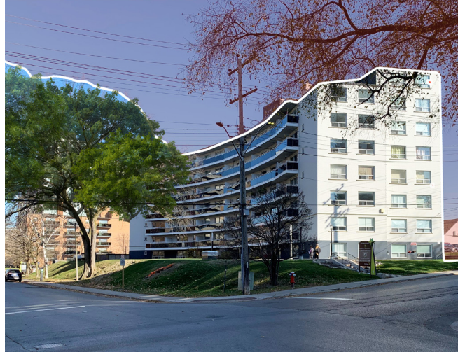
Figure 34: Residential setbacks should be well landscaped. Setbacks should be a minimum of 4.5 m and a maximum of 7.0 m. Mississauga, Mississauga Rd and Bay St
