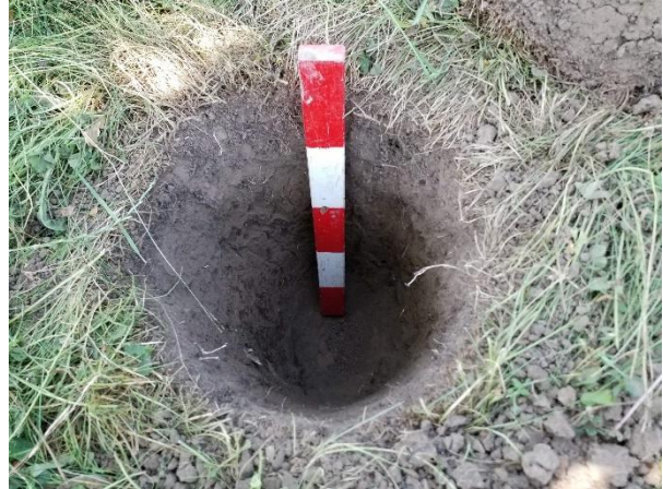
Plate 26: Intact test pit soil profile in the backyard of 5034 Ninth Line. Approximately 20 cm construction fill with a mixed sorting of gravel and concrete debris (Lot 1) overlying 20-25 cm of buried A-horizon (Lot 2) overlying sterile subsoil (B-horizon) (Lot 3).
