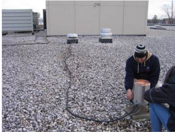
City staff checks in on a tipping bucket rain gauge
