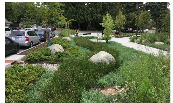
Figure 2.1t-u - Image examples of bioretention cells and rain gardens as an LID approach in park design.
