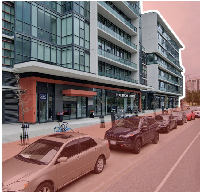
Figure 7: Continuous streetwalls on 'A' frontages are required along the length of a property with provision for articulation and step-back of the streetwall.
