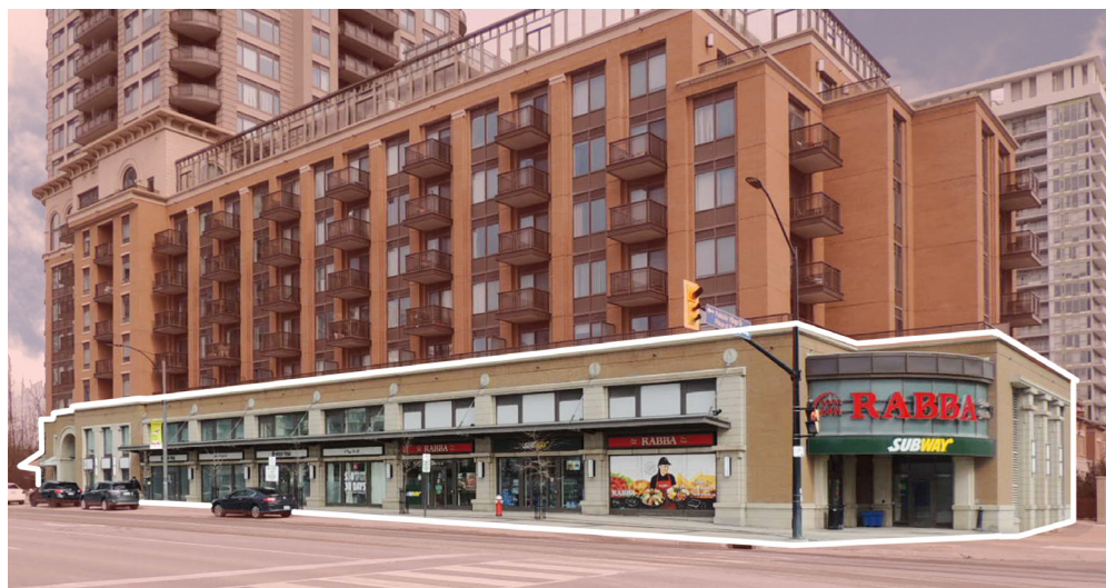
Figure 26: Design the entrances to retail units to a maximum spacing of 10 m between successive storefronts. Downtown Mississauga, Confederation Pkwy & Prince of Wales Dr
