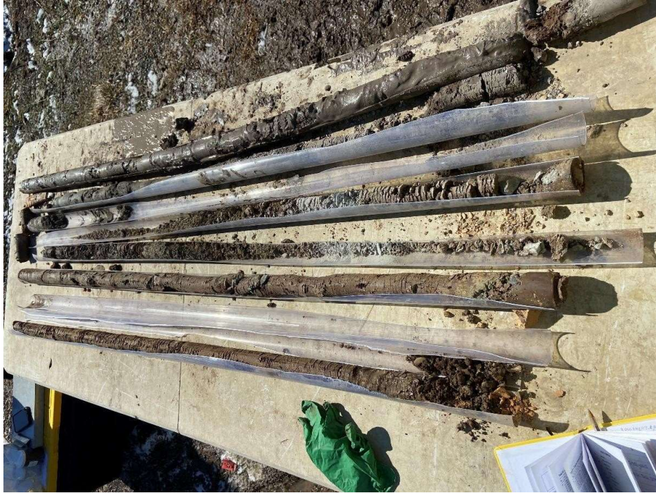
Photo 17: Soil cores extracted from borehole BH8 with Geoprobe continuous core method using Macrocore MC5 dual tube sampling system.
