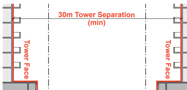
Figure 3: Tower separations and setbacks are measured from the outermost edge of the tower or podium face.
