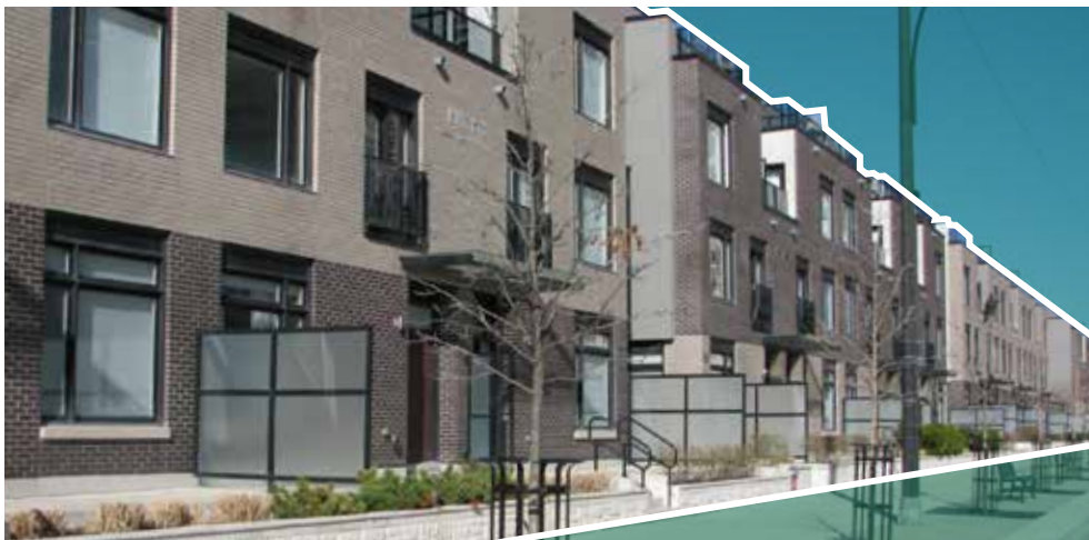
Figure 19: Ground floor conditions on B-Streets. Residential uses are elevated above the ground floor, but directly linked to the public sidewalk through individual points of access serving each unit.
