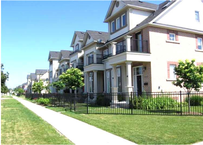
Figure 3.1.4 Preferred —Views to public realm are optimized due to dwellings fronting the street with low open fencing
