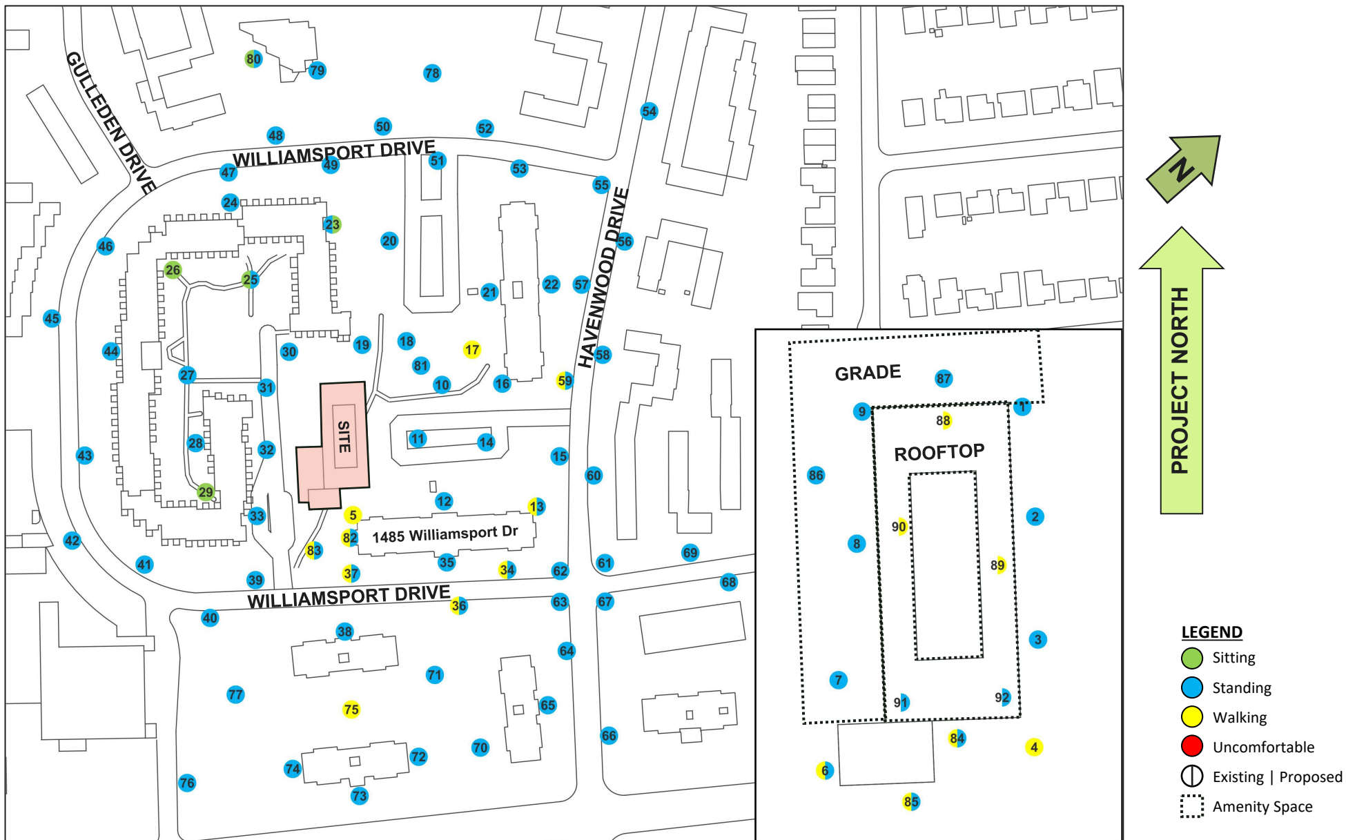
Figure 7: Existing Configuration and Proposed Configuration – Pedestrian Wind Comfort Summer – On-site and Surrounding Areas
