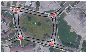
• This alternative modifies the original configuration by placing all-way stop control on both the west and east legs.
