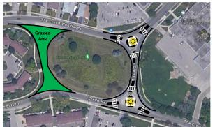
• This alternative modifies the original configuration by closing the west leg and placing mini-roundabouts on the east leg.
