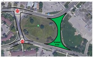
• This alternative modifies the original configuration by closing the east leg and placing all-way stop control on the west leg.
