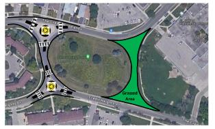
• This alternative modifies the original configuration by closing the east leg and placing mini-roundabouts on the west leg.
