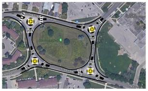
• This alternative modifies the original configuration by placing mini-roundabouts on both the west and east legs.
