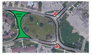
• This alternative modifies the original configuration by closing the west leg and placing one-way stop-controlled T-intersections on the east leg; vehicles on The Credit Woodlands would have right-of-way over vehicles turning from McBride Avenue and Credit Heights Drive.
