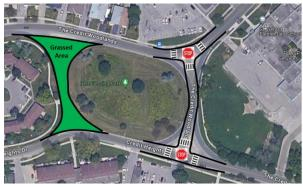
• This alternative modifies the original configuration by closing the west leg and placing all-way stop control on the east leg.
