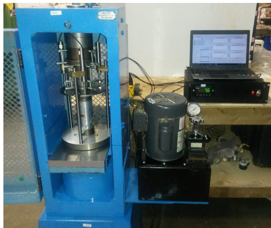
Figure 1: Forney loading frame setup for UCS testing.
