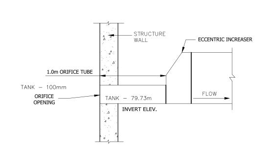
ORIFICE TUBE DETAIL N.T.S.
