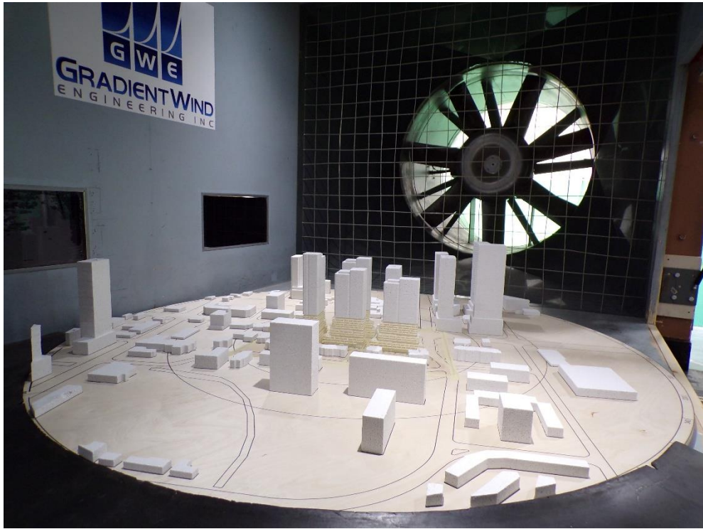
PHOTOGRAPH 9: FUTURE STUDY MODEL INSIDE THE GWE WIND TUNNEL LOOKING DOWNWIND
