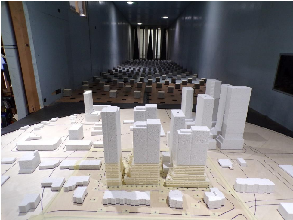
PHOTOGRAPH 10: FUTURE STUDY MODEL INSIDE THE GWE WIND TUNNEL LOOKING UPWIND
