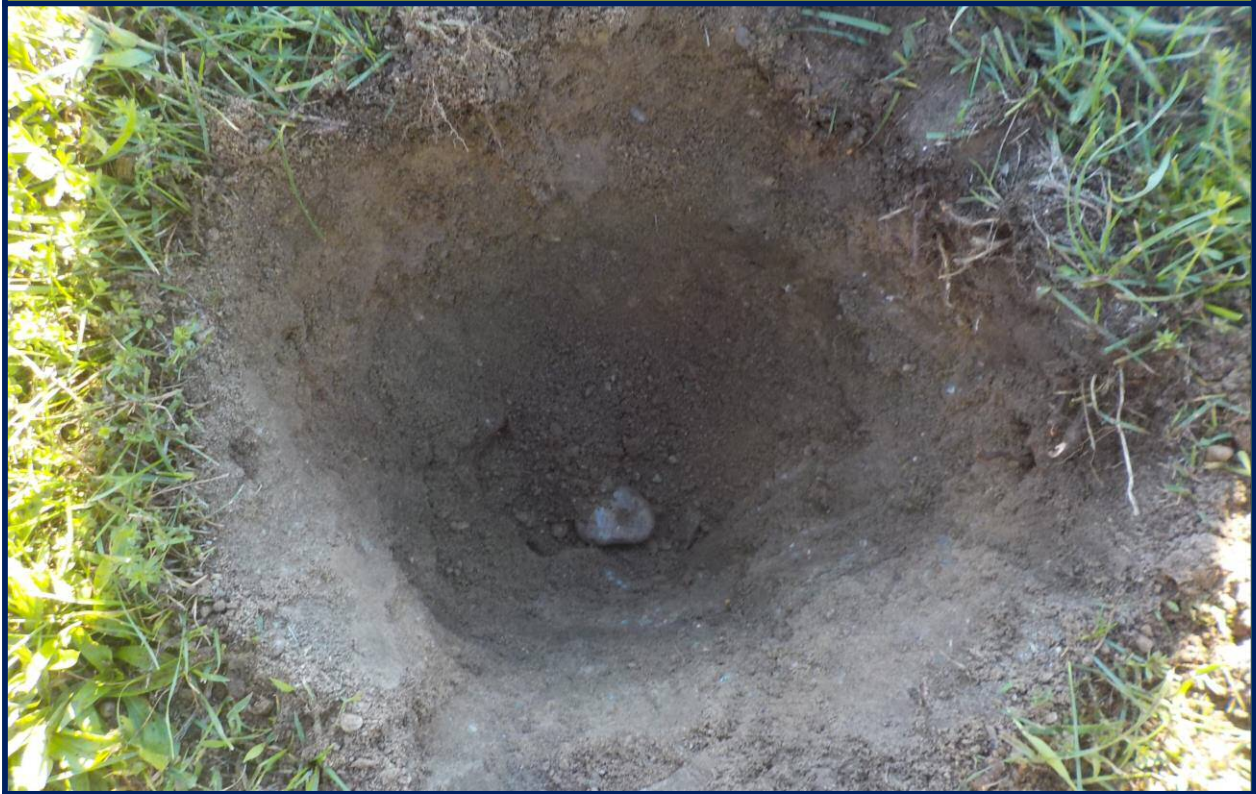
Photo 9: Typical Test Pit from Disturbed Area, Facing South
