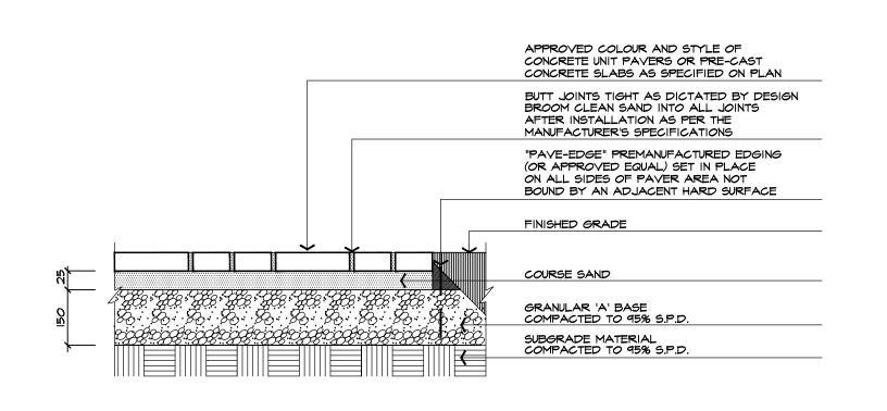
CONCRETE UNIT PAVER DETAIL
