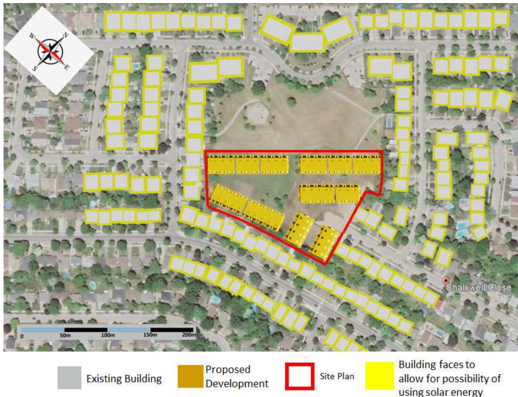
Figure 12: Building Faces in the Vicinity of the Proposed Development
