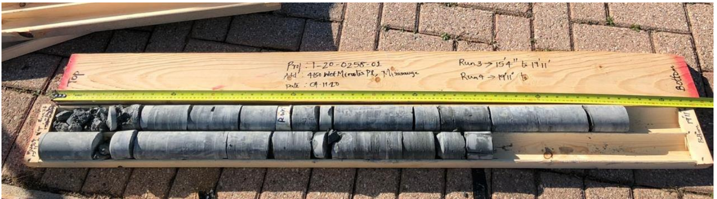
Rock Core Samples – Borehole 1 Runs: 4 & 5 Depth: 6.1 to 8.0 meters
