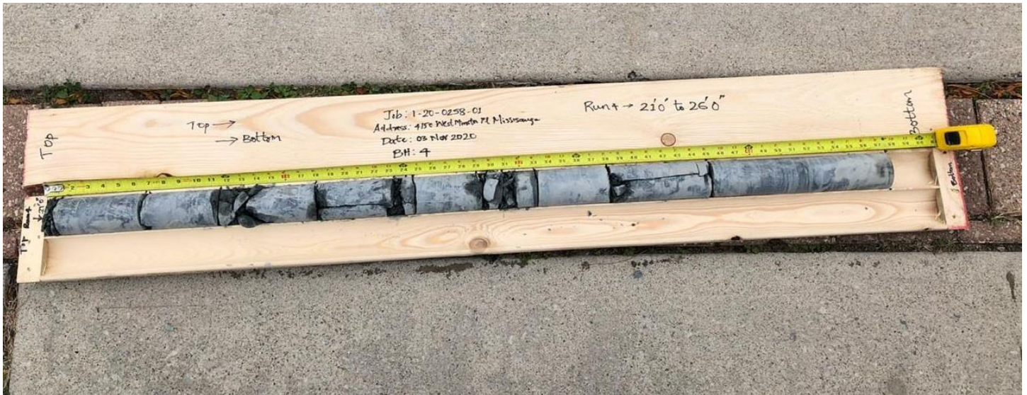
Rock Core Samples- Borehole 4 Runs: 4 Depth: 6.4 to 7.9 meters
