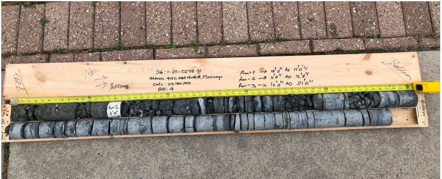
Rock Core Samples- Borehole 4 Runs: 1, 2 & 3 Depth: 3.0 to 6.4 meters
