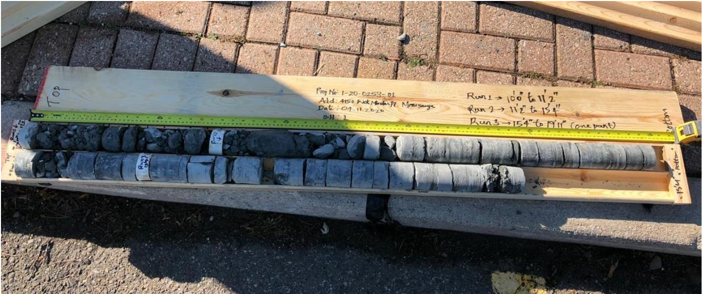
Rock Core Samples- Borehole 1 Runs: 1, 2 & 3 Depth: 3.0 to 6.1 meters
