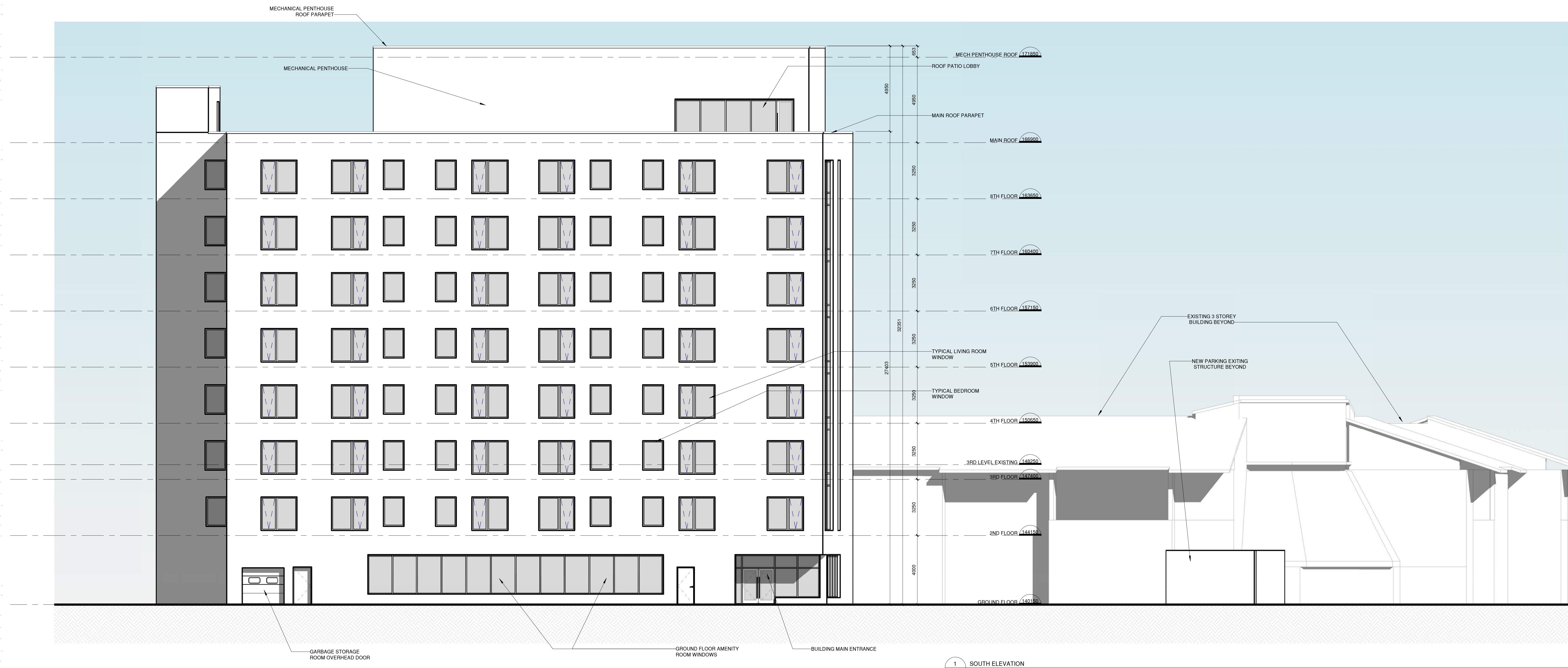
1 SOUTH ELEVATION A401 1:100
