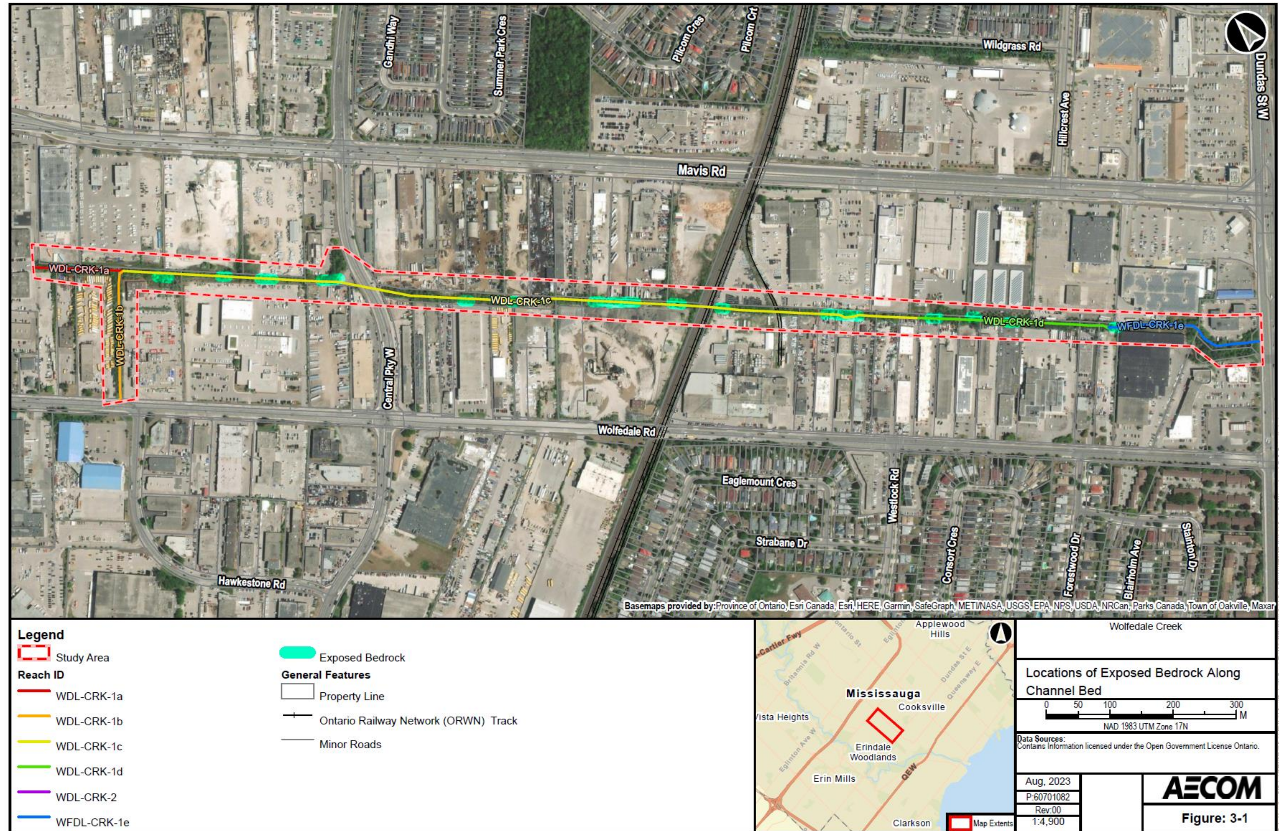
Figure 3-1: Locations of Exposed Bedrock Along Channel Bed – Study Area 1
