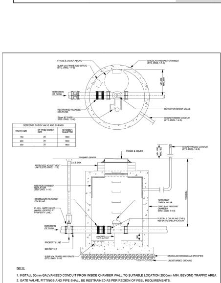
3. ALL PIPING, FITTINGS, VALVES, APPURTENANCES AND MECHANICAL RESTRAINTS TO BE c/w DENSO PASTE, DENSO MASTIC AND DENSO TAPE OR APPROVED EQUAL, APPLIED TO MANUFACTURER'S RECOMMENDATIONS.
