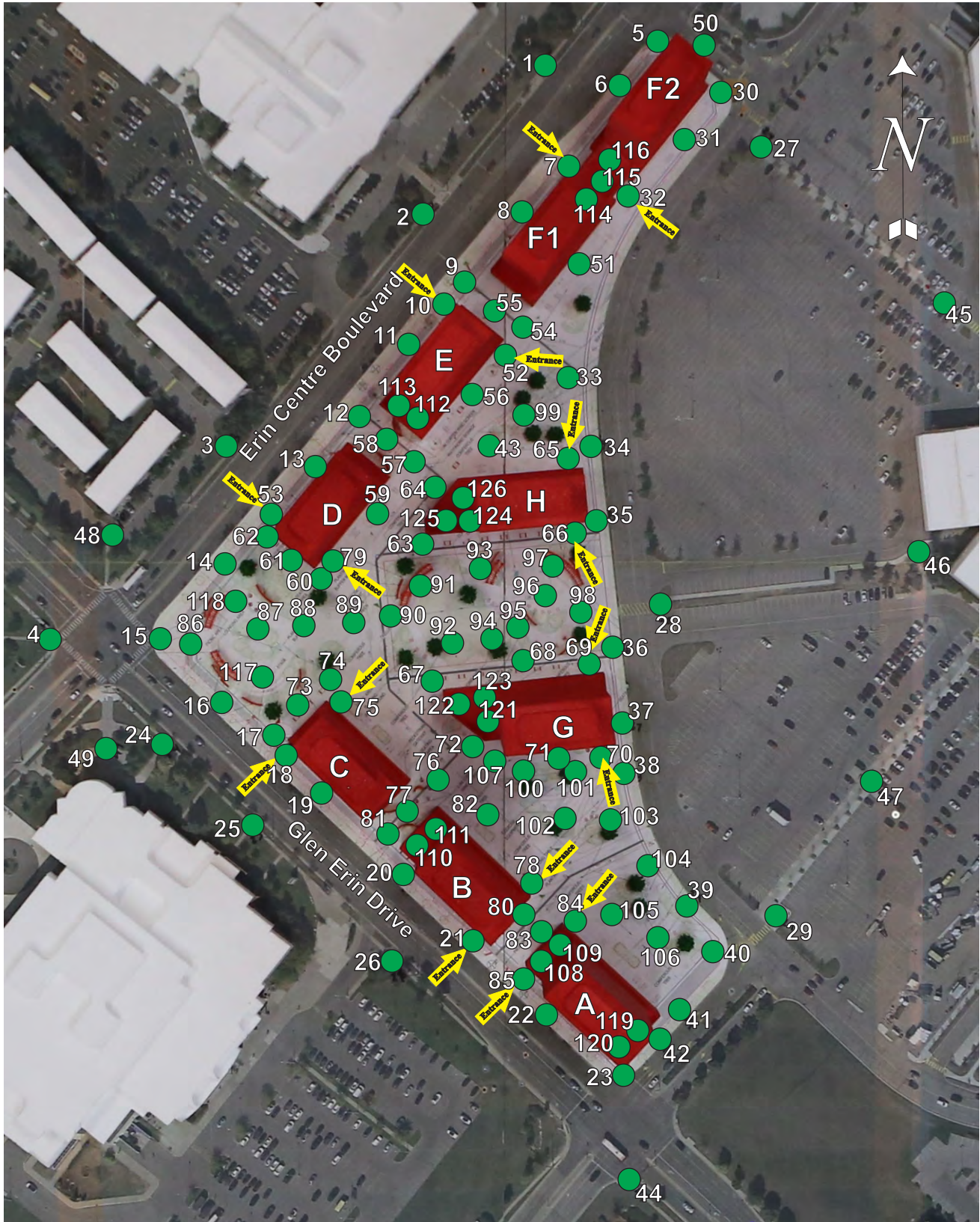
Figure 4: Location Plan for Pedestrian Level Wind Velocity Measurements 27
