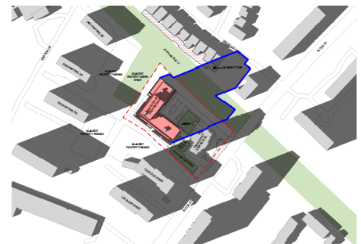
SEPTEMBER 21 AT 17.12 1 : 1600 TOTAL SHARED OUTDOOR AMENITY AREA: 1327m 2 AREA IN SUNSHINE AT THIS TIME: 75m 2
