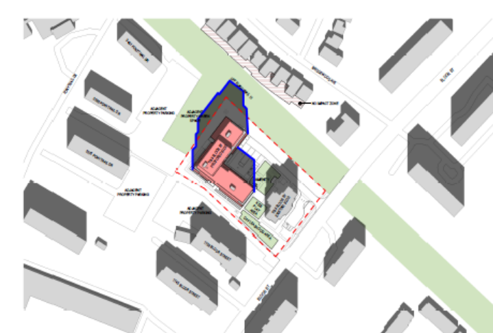
SEPTEMBER 21 AT 13.12 1 : 1600 TOTAL SHARED OUTDOOR AMENITY AREA: 1327m 2 AREA IN SUNSHINE AT THIS TIME: 1085m 2
