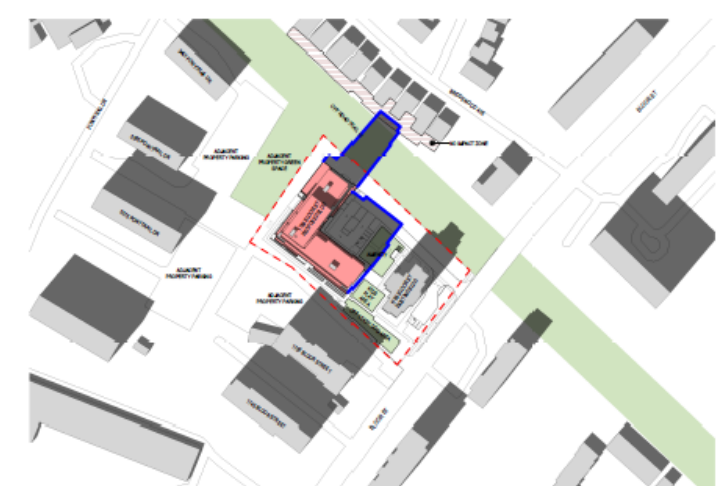
SEPTEMBER 21 AT 15.12 1 : 1600 TOTAL SHARED OUTDOOR AMENITY AREA: 1327m 2 AREA IN SUNSHINE AT THIS TIME: 827m 2
