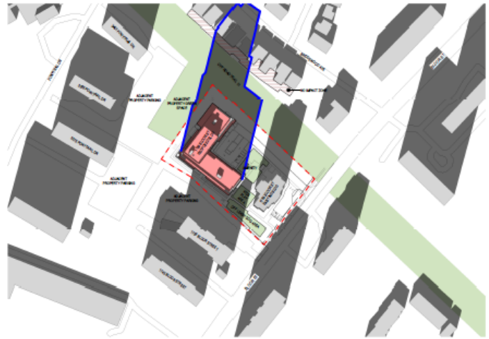
DECEMBER 21 AT 13.17 1: 1600 TOTAL SHARED OUTDOOR AMENITY AREA: 1327m 2 AREA IN SUNSHINE AT THIS TIME: 750m 2
