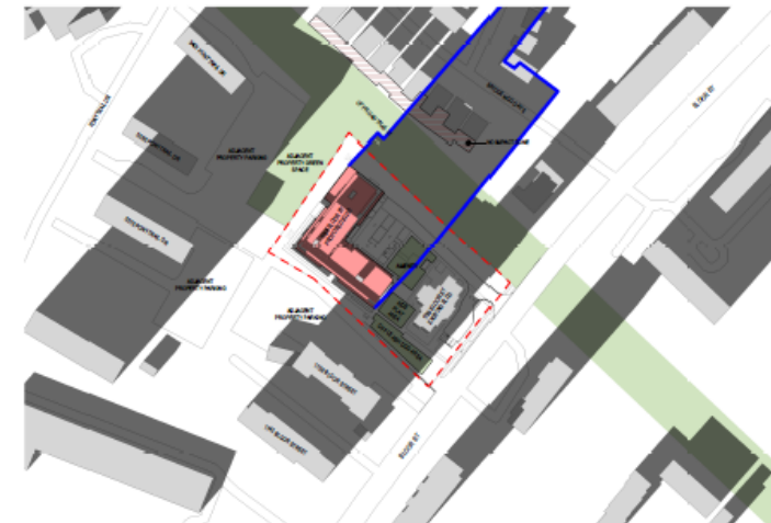
DECEMBER 21 AT 15.15 1: 1600 TOTAL SHARED OUTDOOR AMENITY AREA: 1327m 2 AREA IN SUNSHINE AT THIS TIME: 22m 2
