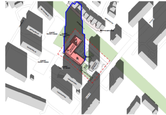
DECEMBER 21 AT 12.17 1: 1600 TOTAL SHARED OUTDOOR AMENITY AREA: 1327m 2 AREA IN SUNSHINE AT THIS TIME: 871m 2
