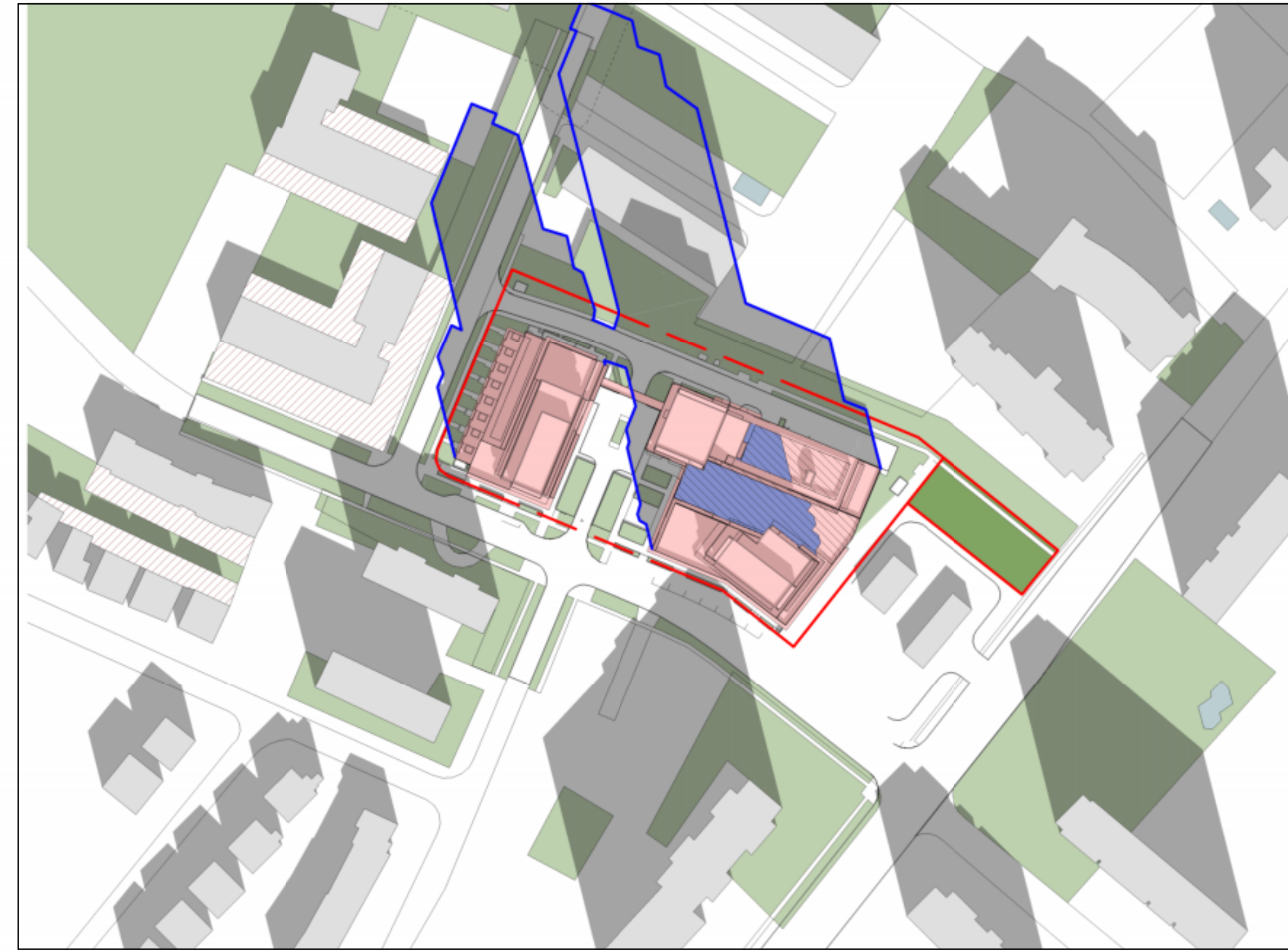
DECEMBER 21 AT 10.17 1 : 1600 TOTAL SHARED OUTDOOR AMENITY AREA: 1,927 m 2 TOTAL AREA OF SUNSHINE AT THIS TIME: 732 m 2 AMENITY LEVEL 2: 382 m 2 AMENITY LEVEL 6: 350 m 2
