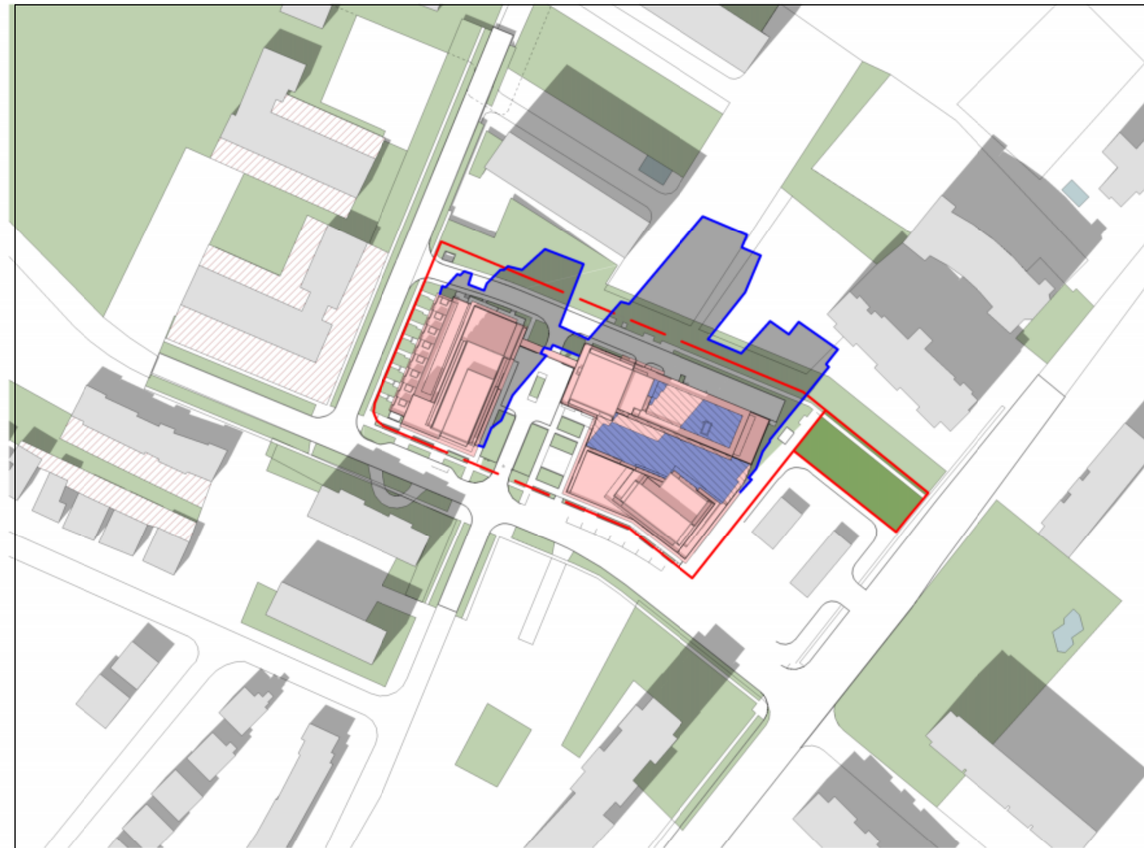
SEPTEMBER 21 AT 14.12 1 : 1600 TOTAL SHARED OUTDOOR AMENITY AREA: 1,927 m 2 TOTAL AREA OF SUNSHINE AT THIS TIME: 540 m 2 AMENITY LEVEL 2: 292 m 2 AMENITY LEVEL 6: 248 m 2
