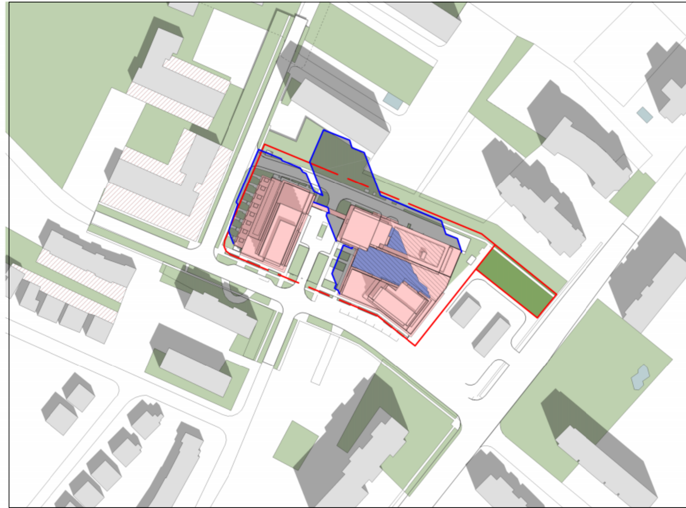
SEPTEMBER 21 AT 11.12 1 : 1600 TOTAL SHARED OUTDOOR AMENITY AREA: 1,927 m 2 TOTAL AREA OF SUNSHINE AT THIS TIME: 936 m 2 AMENITY LEVEL 2: 469 m 2 AMENITY LEVEL 6: 467 m 2
