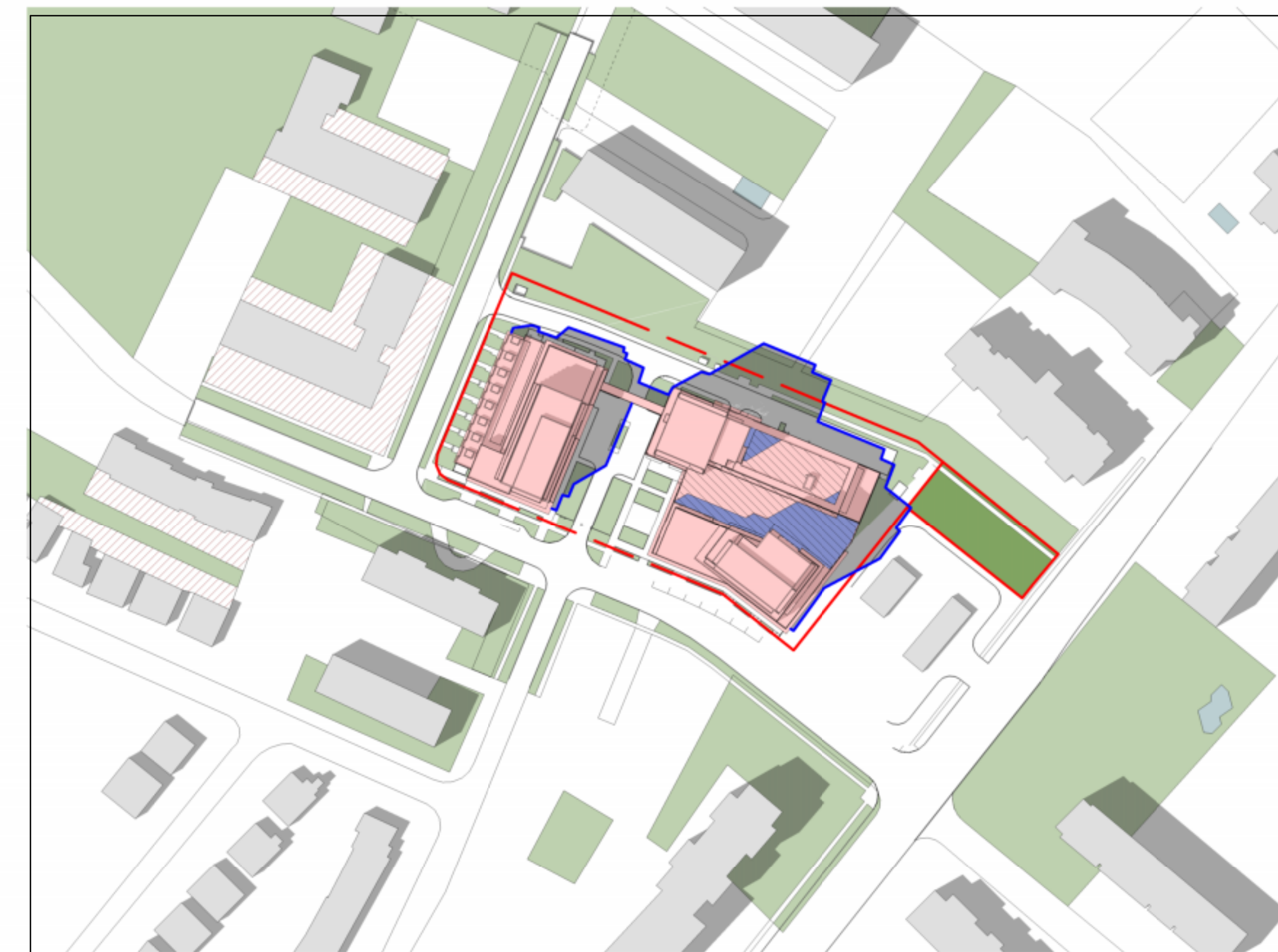
JUNE 21 AT 14.20 1 : 1600 TOTAL SHARED OUTDOOR AMENITY AREA: 1,927 m 2 TOTAL AREA OF SUNSHINE AT THIS TIME: 1,113 m 2 AMENITY LEVEL 2: 609 m 2 AMENITY LEVEL 6: 504 m 2
