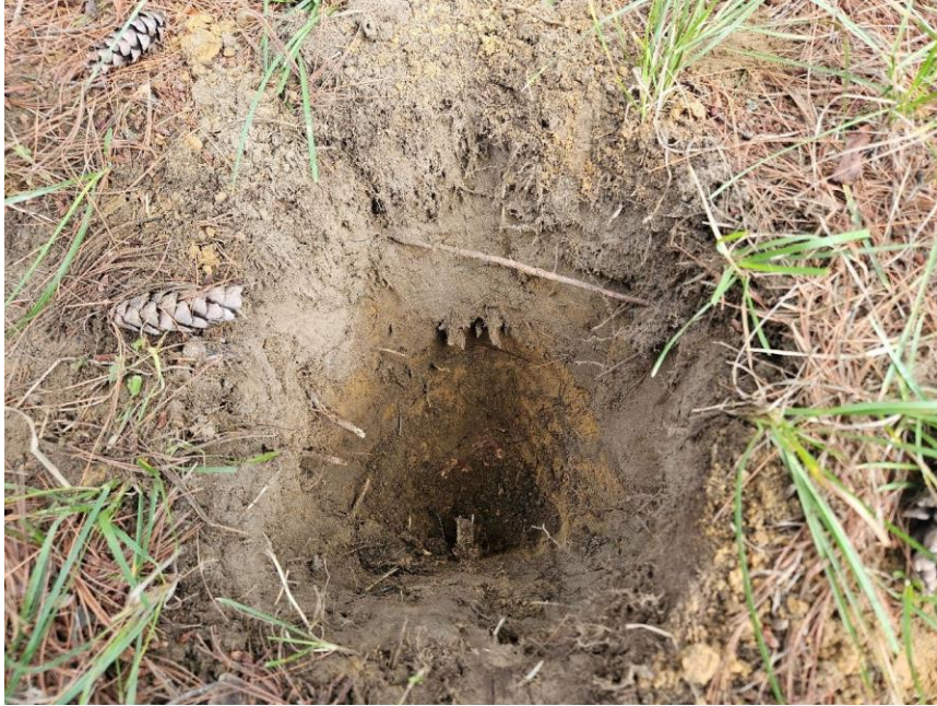
Image 5: View of typical test pit soil profile.
