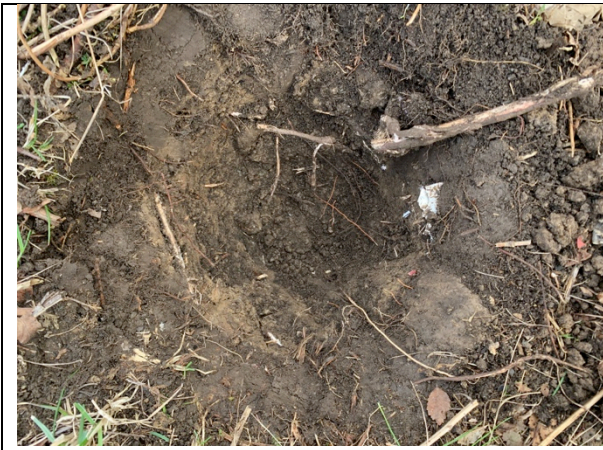
IMAGE 1 DISTURBED TEST PIT WITH FILL LAYER
