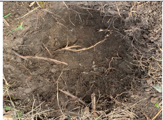
IMAGE 2 TEST PIT IN PROGRESS WITH FILL LAYER
