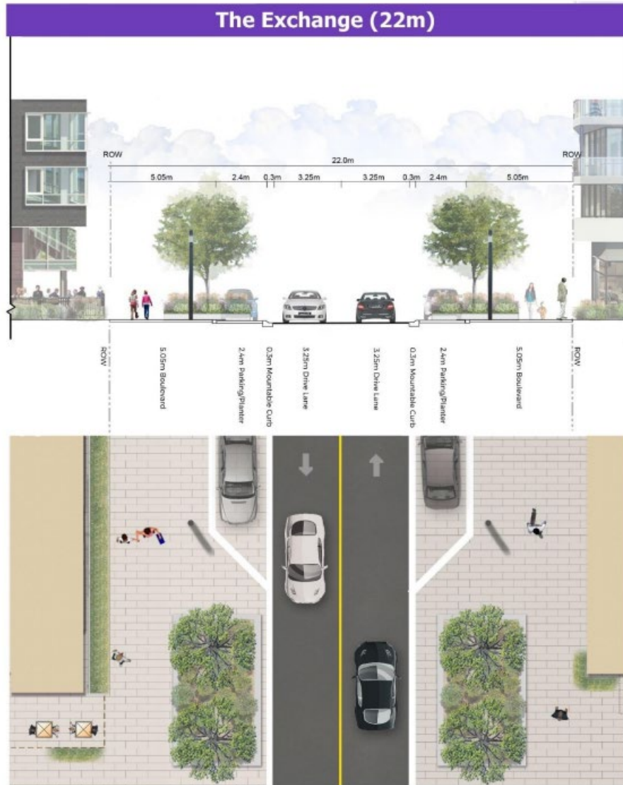
Figure 2-19: Preferred The Exchange Cross-section
