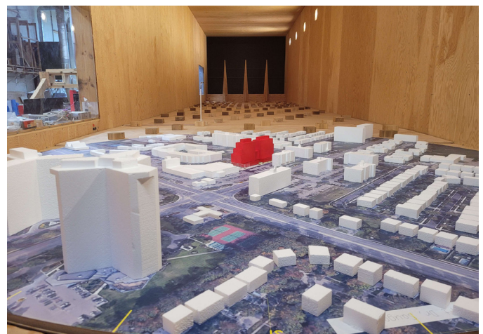
Figure 24 - Wind Testing Facility (Source: Theakston)
